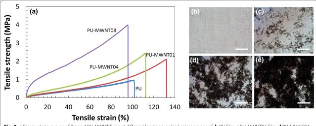
Fig. 3 a Stress-strain curves of PU and PU-MWNT films at different loadings, optical micrographs of; **b** PU film, **c** PU-MWNT01 film, **d** PU-MWNT04 film, and **e** PU-MWNT08 film. *Scale bars* represent 100 μm
