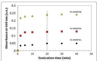
**Fig. 1** Effect of increasing sonication time on the UV–visible absorption spectrum at 600 nm of palm kernel oil-polyester (PKO-p) dispersion containing 0.01 wt. %, 0.04 wt. %, and 0.08 wt. % MWNTs
