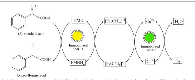
**Fig. 1** Bi-enzymatic system with immobilized SMDH and immobilized laccase catalyzed continuously the transformation of (S)-mandelic acid to benzoylformic acid using ferricyanide/ferrocyanide as the redox medium
