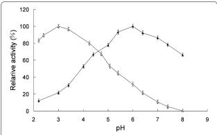
**Fig. 3** Effects of pH on free and immobilized laccase activities. *Open triangle* indicated soluble laccase, and *close triangle* indicated immobilized laccase. Reactions were performed in triplicate, and *error bars* represented standard deviations (StDev)
