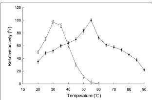
**Fig. 4** Effects of temperature on free and immobilized laccase activities. *Open circle* indicated soluble laccase, and *close circle* indicated immobilized laccase. Reactions were performed in triplicate, and *error bars* represented standard deviations (StDev)
