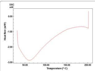
**Fig. 8** DSC heating curve of *Chlorella pyrenoidosa* protein concentrate by TPP
