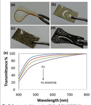
**Fig. 2** Photograph of the sample; **a** PU film, **b** PU-MWNT01 film, **c** PU-MWNT04 film, **d** PU-MWNT08 film, and **e** decreased transmittance (%) of PU film at higher loading of MWNTs
