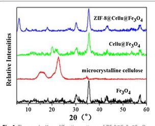
**Fig. 1** The powder X-ray diffraction patterns of ZIF-8@Cellu@Fe<sub>3</sub>O<sub>4</sub>, Cellu@Fe<sub>3</sub>O<sub>4</sub>, and microcrystalline cellulose
