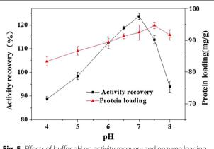
**Fig. 5** Effects of buffer pH on activity recovery and enzyme loading of immobilized GOx
