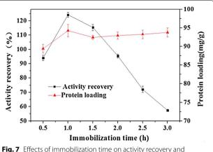
**Fig. 7** Effects of immobilization time on activity recovery and enzyme loading of immobilized GOx
