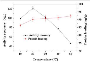
**Fig. 6** Effects of immobilization temperature on activity recovery and enzyme loading of immobilized GOx
