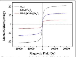
**Fig. 4** Hysteresis loops of Fe $_3$ O $_4$ , Cellu@Fe $_3$ O $_4$ , ZIF-8@Cellu@Fe $_3$ O $_4$ , and GOx-ZIF-8@Cellu@Fe $_3$ O $_4$
