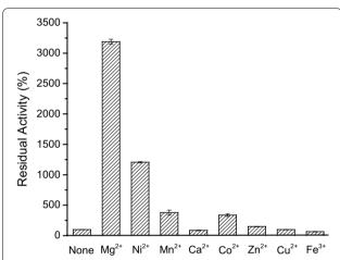
**Fig. 3** Effects of cations on the specific activity of AfPase. The reactions were performed in 100 mM HEPES buffer (pH 7.0) containing 1 mM *p*-nitrophenyl phosphate, 5 mM different ions, and appropriate concentration of phosphatase at 85 °C
