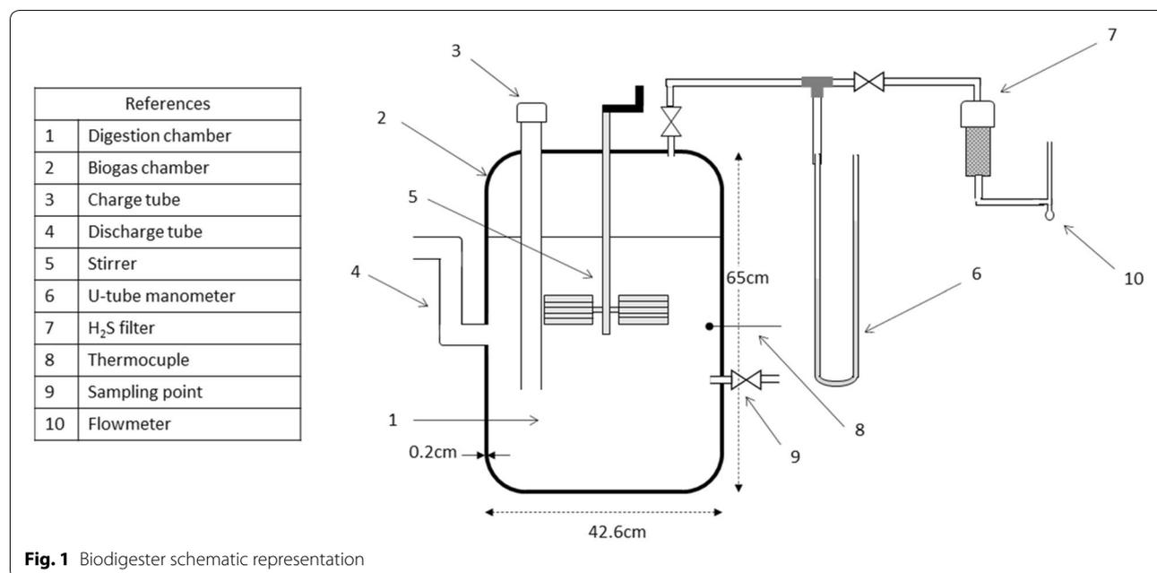
**Fig. 1** Biodigester schematic representation
