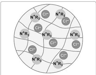
**Fig. 3** Schematic anion-exchange resin beads. By permission from Rohm and Haas, Inc., Pennsylvania, United States (Rohm and Haas 2008)
