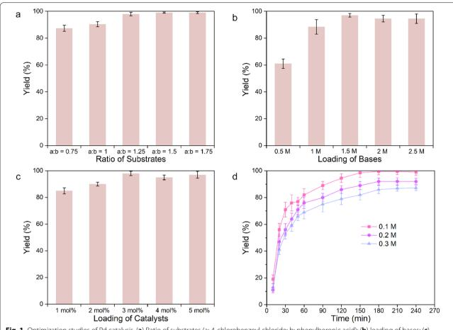
Fig. 1 Optimization studies of Pd catalysis. (a) Ratio of substrates (a: 4-chlorobenzoyl chloride; b: phenylboronic acid); (b) loading of bases; (c) loading of catalysts; (d) reaction time and different concentrations of substrates of 4-chlorobenzoyl chloride
