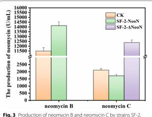
**Fig. 3** Production of neomycin B and neomycin C by strains SF-2, SF-2-NeoN, and SF- $2\Delta$ NeoN during fermentation
