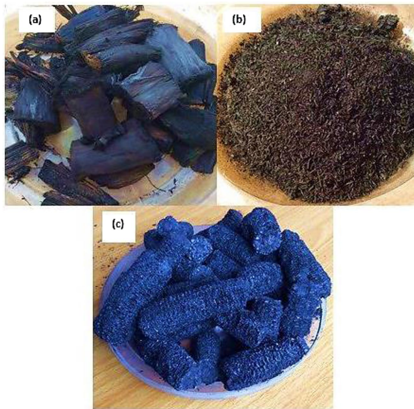
Fig. 4 Biochar samples generated from (a) banana stalk, (b) rice husk, and (c) corncob. Adopted from Ibitoye et al. (2022) and modified (Open access without copyright permission requirement)
