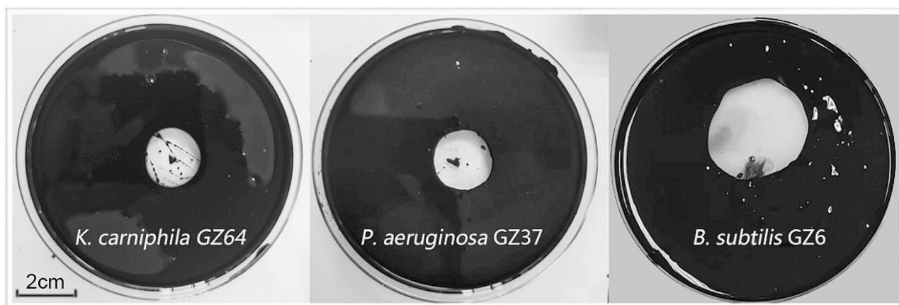
Fig. 1 Positive strains in the oil spreading test. Average diameters of oil discharge rings: Kocuria carniphila GZ64, 1.7 \pm 0.1 cm, Pseudomonas aeruginosa GZ37, 1.9 \pm 0.1 cm, and Bacillus subtilis GZ6, 3.5 \pm 0.2 cm; Each experiment was performed in triplicate
