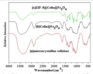
**Fig. 2** FT-IR spectra of microcrystalline cellulose (**a**), Cellu@Fe $_3$ O $_4$  (**b**), and ZIF-8@Cell@Fe $_3$ O $_4$  (**c**).
