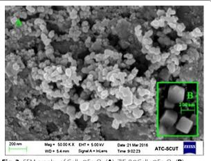
Fig. 3 SEM graphy of Cellu@Fe<sub>3</sub>O<sub>4</sub> (A), ZIF-8@Cellu@Fe<sub>3</sub>O<sub>4</sub> (B)
