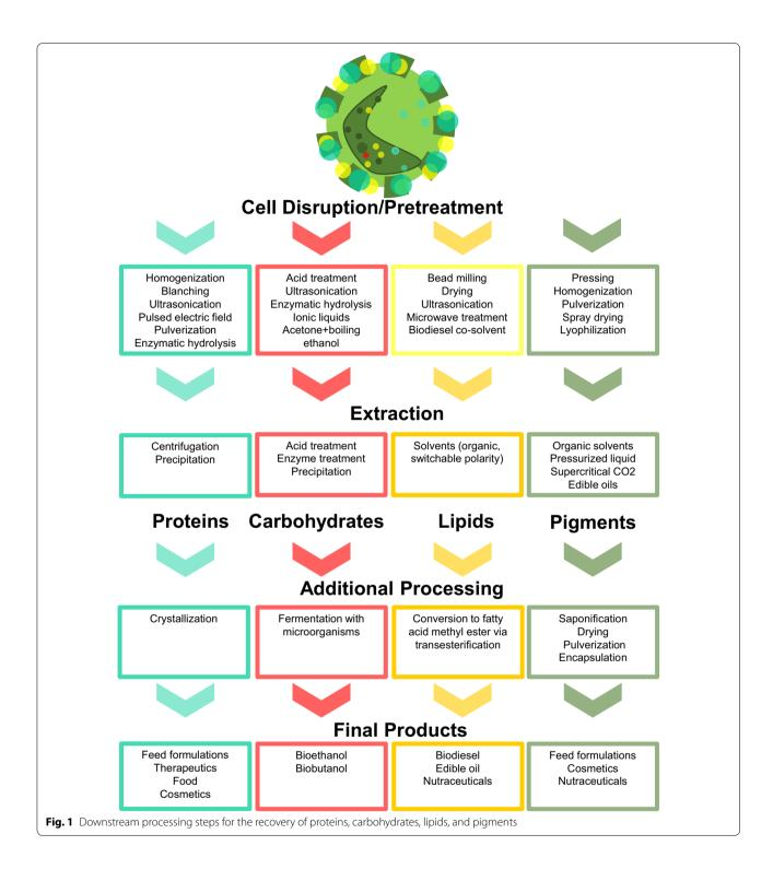
depending on the characteristics of the microalgae cell wall/membrane and target molecules. Mechanical cell disruption methods include bead beating, high pressure homogenization (HPH), high speed homogenization (HSH), ultrasonication, and pulsed electric field (PEF)
