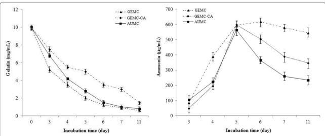
**Fig. 2** Effect of incubation time on the degradation of gelatin (left) and liberation of ammonia (right) by enriched methanogenic cultures in anaerobic batch digestion (*AUMC* acetate-utilizing methanogenic culture, *GEMC* gelatin-enriched mixed culture, *GEMC-CA* gelatin-enriched mixed culture with *Clostridium acetobutylicum* NCIM 2841)
