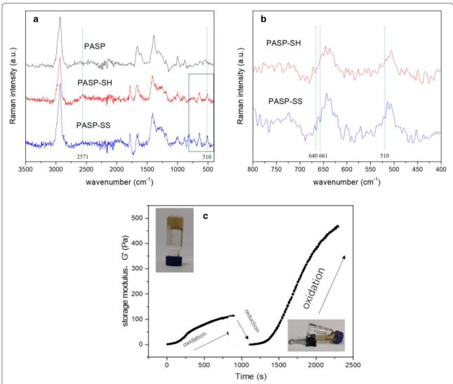
**Fig. 1** Raman spectra and sol–gel transition of PASP-SH and PASP-SS. **a** Raman spectra of PASP, reduced state PASP-SH and oxidised state PASP-SS; **b** detailed spectra of PASP-SH and PASP-SS in the range of 400–800 cm<sup>-1</sup>; **c** rotating rheology measurement of reversible redox-induced sol–gel transition of PASP-SH; the upper left illustration shows oxidised PASP-SS gel, and the lower right illustration shows reduced PASP-SH sol
