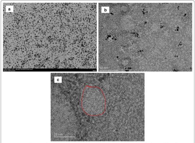
Fig. 2 TEM images of PtNPs a and PtNPs-ProK b, c at different scales, where b, c sample was negatively dyed, c the shape inside the red line is ProK
