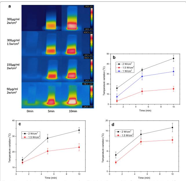
Fig. 4 NIR-triggered photothermal conversion and enzyme release of PtNPs-ProK. a Thermographs by infrared laser on PtNPs-ProK under different contents of PtNPs and different infrared power densities; effect of different infrared power densities on temperature changes of PtNPs-ProK solution at a concentration of 300 μg/mL PtNPs (b), 150 μg/mL PtNPs (c), and 50 μg/mL PtNPs (d)
