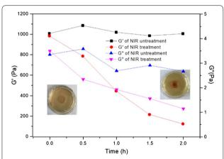
**Fig. 6** Storage modulus *G'* and loss modulus *G''* of H-PtNPs-ProK with time; the left-hand photograph shows H-PtNPs-ProK without irradiation: the right-hand photograph shows H-PtNPs-ProK after 2 h of NIR irradiation
