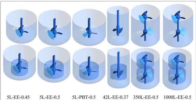
**Fig. 1** Schematic diagram of the three-dimensional bioreactors and impeller zones for CFD simulation (the text at the bottom indicates the type of each bioreactor, namely, "bioreactor volume-impeller type-ratio of impeller diameter to tank diameter")
