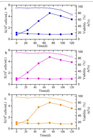
**Fig. 6** Viable cell density (*X*, filled square), viability (triangle), and the ratio of aggregated cells (*A*, filled circle) in batch cultures of BHK-21 cells in 42- (**a**), 350- (**b**), and 1000-L (**c**) bioreactors
