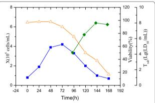
**Fig. 7** Viable cell density (X, filled square), viability (triangle), and virus titer ( $T_{\rm rab}$ , filled diamond) in the batch culture of BHK-21 cells in the 1000-L bioreactor
