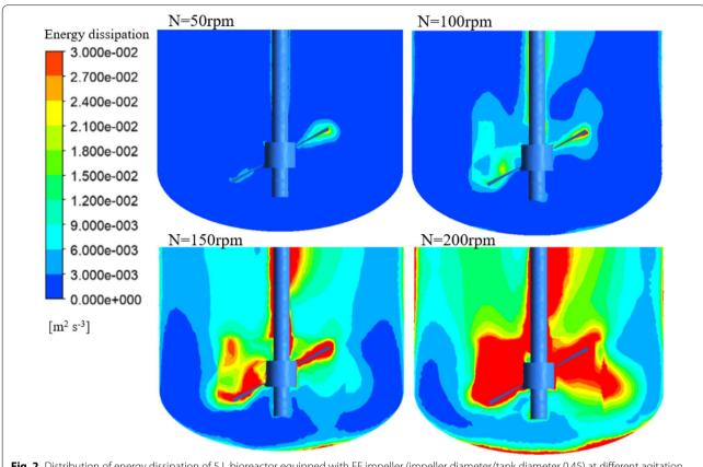
Fig. 2 Distribution of energy dissipation of 5 L bioreactor equipped with EE impeller (impeller diameter/tank diameter 0.45) at different agitation speeds
